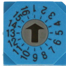
Figure 24: Rotary Switch Address Settings
